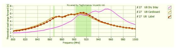
Sensitivity&Read Range Test power: 4W EIRP
